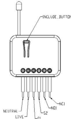
device and is fully compatible with any Z-Wave™ enabled network. Slim design let the Controller can easily hide itself into the wall box and that will be good for the house decoration.
